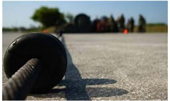
The arrestor gear cable with 'fishing floats' at Kadena.
